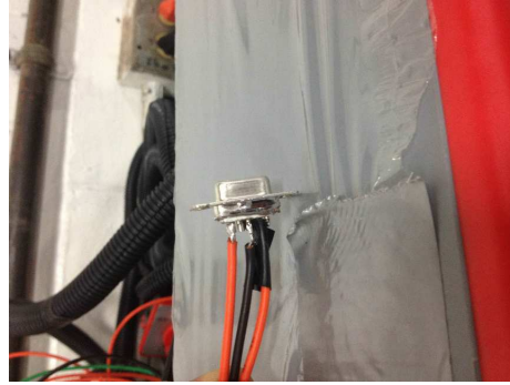
Figure B.10: RS232 wire used for communicating with the charger cub-controller.
