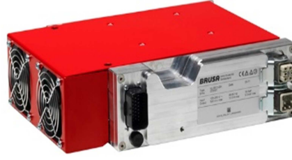
Figure B.9: BRUSA NLG514 3.3 kW battery charger.
